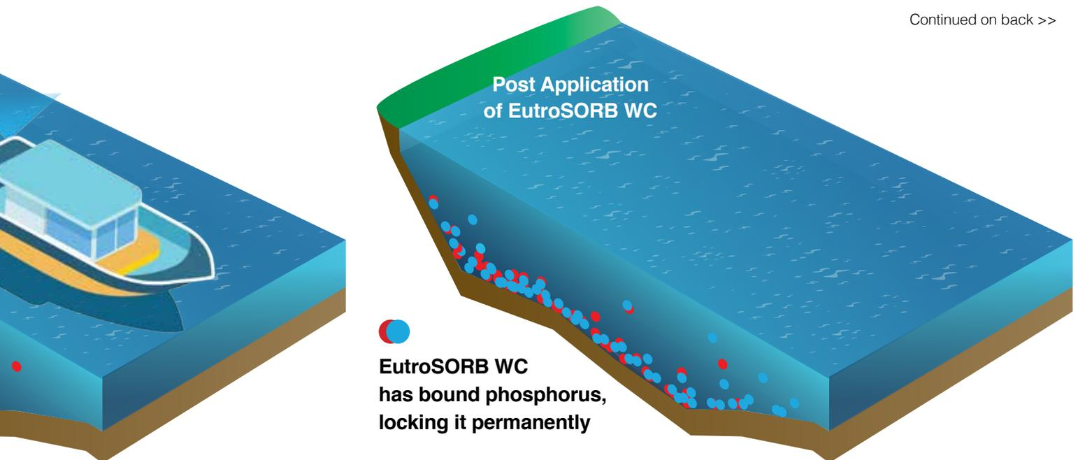
phosphorus inactivation. When making applications to flowing water (e.g., rivers, streams, canals, ditches, etc.), inject, drip, or pour EutroSORB WC at a location where adequate mixing occurs to optimize phosphorus binding.
